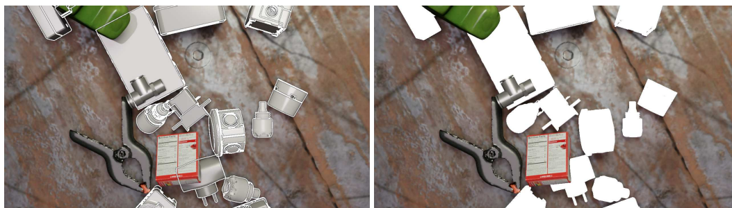
Figure 2: A Sample of a T-LESS Training Scene with Overlaid Target Object Edges on the Left and Visibility Masks on the Right
