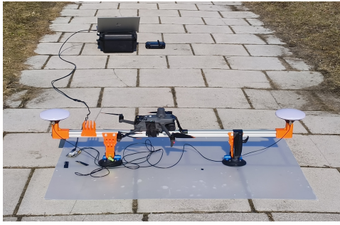
(a) Heading (Yaw)-accuracy of the drone
