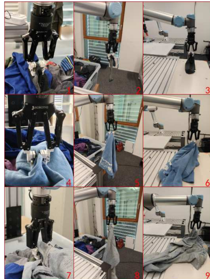
(b) Garment manipulation process, showcased on a sock 1-3, a shirt 4-6 and a trouser 7-9. The first image displays a textile being grasped from the box, the second image displays the textile in the air and the third image displays the textile being placed on the inspection table.
