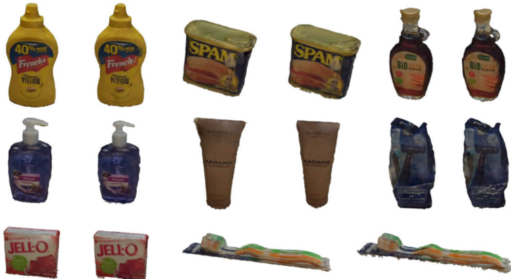
Figure 5: Overview of the reconstruction quality of objects that are used in the grasp evaluation. For each pair, the left mesh is from 2DGS and the right from SVRaster.
