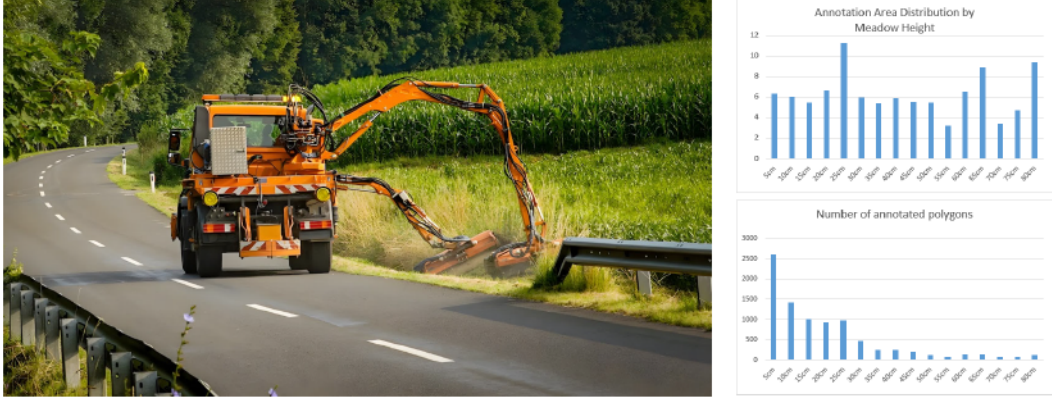
Figure 1: Road maintenance service vehicle from the province of Styria during mowing activity (left). Statistical breakdown of the annotated dataset (right). The histograms show a comparison between total annotated area (top) and polygon counts (bottom) across 5 cm height increments.
