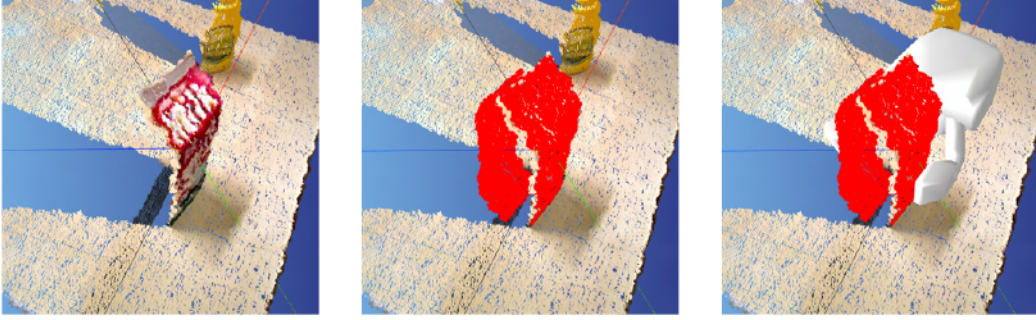
(a) The original point cloud in real coloring with the blue ray being the view ray direction. (b) The fully augmented point cloud in red with the symmetry-based added part. (c) The chosen grasp based on the augmented point cloud.
